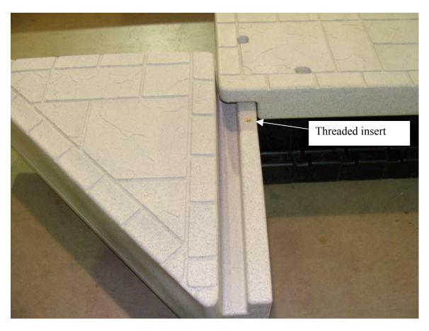
2. Slide the corner gusset section down the H-channel until it butts up to the adjoining dock section. The threaded insert in the gusset should line up with the hole in the dock deck. Secure with the  $3/8 \times 1 \frac{1}{2}$  bolt and washer. A simple L-shaped dock assembly is shown.
