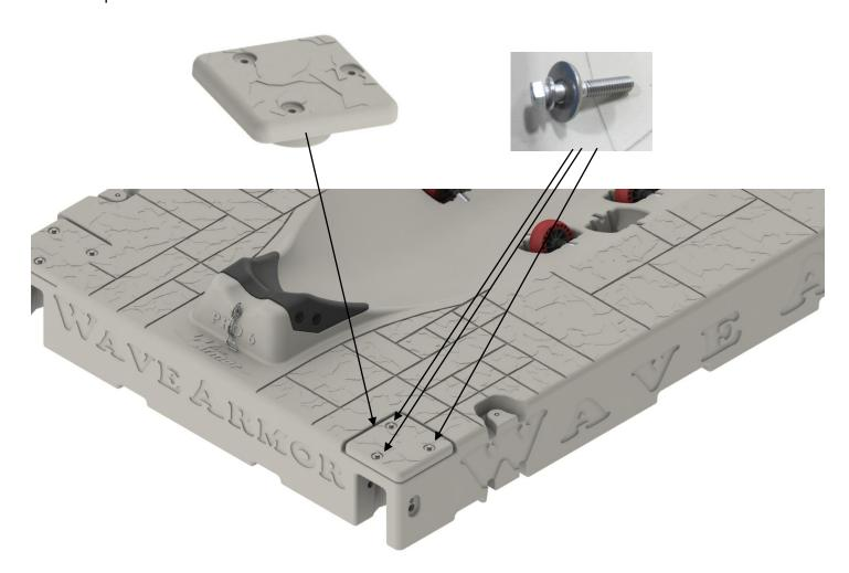
2. Caps may also be installed at the rear of the port. The procedure is the same.
