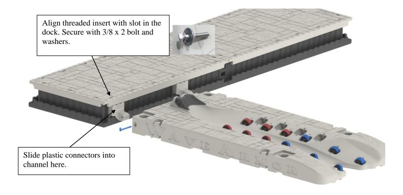
2. Align port with the two plastic connectors. Push the port forward so it can be connected to the dock. Insert connector pin through the port and through the hole in the plastic connector. Secure connector pin with the 3/8 shoulder bolt and thin washer. Repeat on the other side. Tighten securely with the allen wrench.
