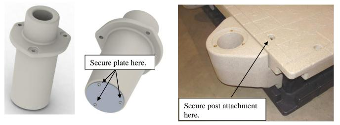
3. Insert flag pole sleeve into the opening on the dock post attachment. Secure with the  $3/8 \times 1 \frac{1}{4}$ " bolts and 3/8 washers. Insert flag pole into the sleeve. Will fit flag poles up to  $2 \frac{1}{2}$ " outside diameter.
