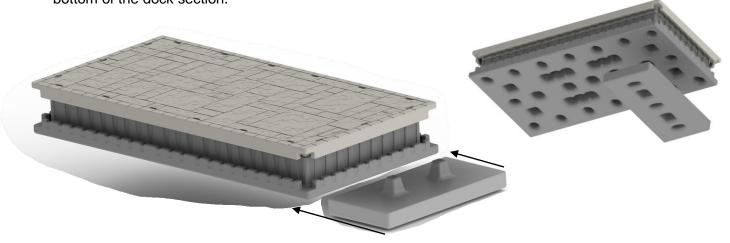
2. Push the booster under the water and under the dock section until the tabs lock into the dock.
