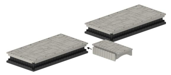
2. Once the bridge section is in place, insert an oval washer into the two center slots and secure with the 3/8 x 2 bolts and lock washers. Install the remaining bolts, heavy washers and lock washers into the other 4 slots in the dock. Tighten securely.
